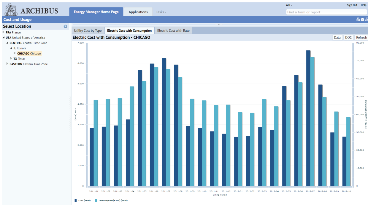
Graphical dashboard views, such as Utility Cost with Consumption (by building and billing period) shown above, simplifies visualization and analysis while improving decision support for energy management strategies
